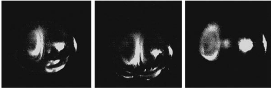
FIGURE 3. Single video frames displaying the light scattered from a trapped air bubble containing suspended tracer particles. A steady-state streaming flow can be observed within the air bubble. The velocity distribution is highly non-uniform because the principal driving mechanism for streaming appears to be the capillary waves at the bubble top surface.
